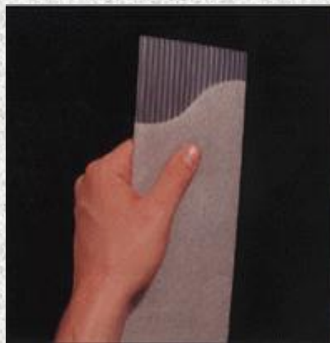
Fig. 1 Typical Prefabricated Vertical Drain (PVD)
